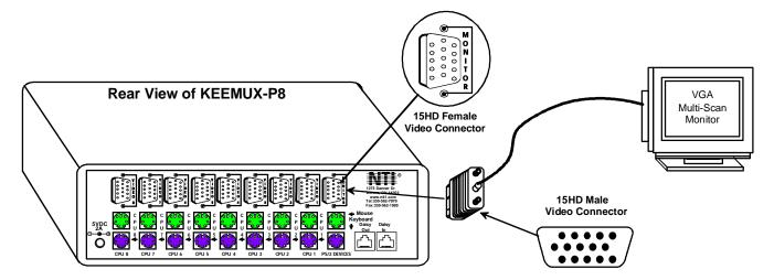
Figure 2- Connect the monitor to the KEEMUX
